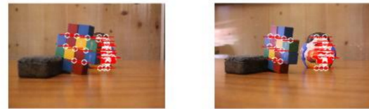
Figure 9: SIFT matching points we find for experiment 1. The red lines are the epipolar lines at each point.
