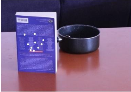
Figure 25: Re-projection result for experiment 3; White points are SIFT points that are re-projected back. There are no yellow points on this graph as we use ratio instead of symmetry approximation.
